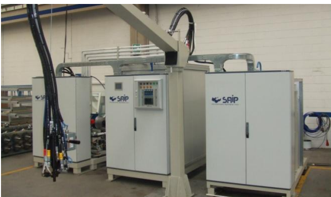
Photo: foam dispensing equipment that is able to use a premixed Polyol / HC blend along with the option to metering HC as third stream directly into a mixing and pouring head.
